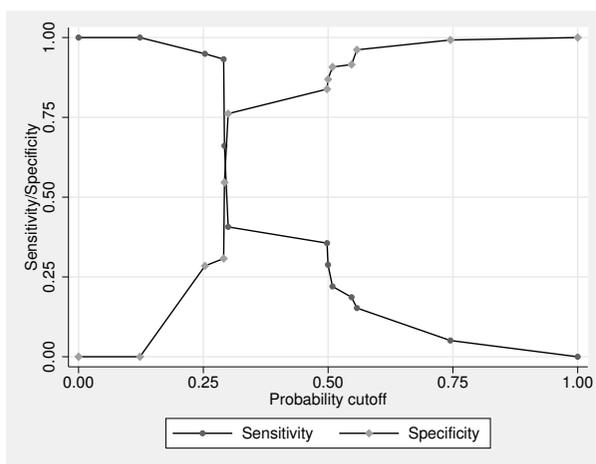
`lsens` optionally creates new variables containing the probability cutoff, sensitivity, and specificity.
