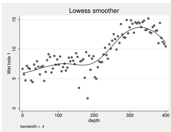
In the first case, the default bandwidth of 0.8 is used, meaning that 80% of the data are used in smoothing each point. In the second case, we explicitly specified a bandwidth of 0.4. Smaller bandwidths follow the original data more closely.
