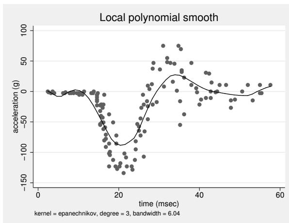
The default bandwidth and kernel settings do not provide a satisfactory fit in this example. To improve the fit, we can either supply a different bandwidth by using the `bwidth()` option or specify a different kernel by using the `kernel()` option. For example, using the alternative Epanechnikov kernel, `kernel(epan2)`, below provides a better fit for these data.
