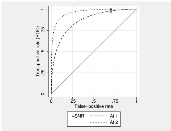
At the higher false-positive rate value of 0.7, we see little difference in the ROC values and note that the confidence intervals nearly overlap. Now we view the same curves with the lower false-positive rate compared.
