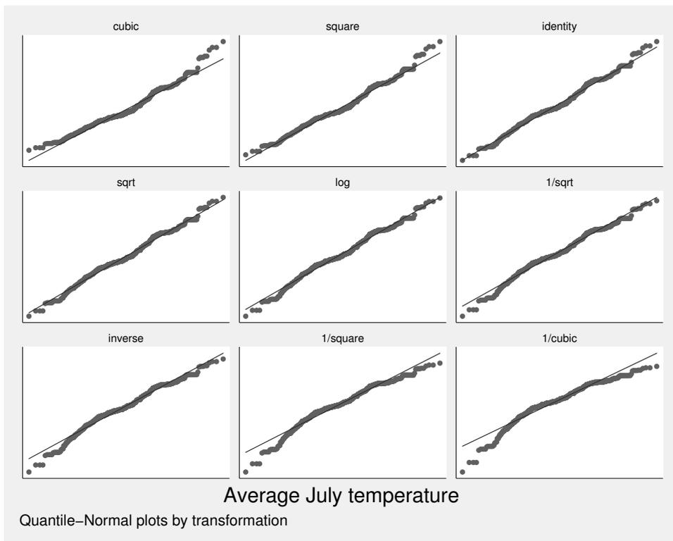
This graph shows that for the square transform, the upper tail—and only the upper tail—diverges from what would be expected. This divergence is detected by `sktest` (see [R] [sktest](#)) as a problem with skewness, as we would learn from using `sktest` to examine `tempjuly` squared and square rooted.
