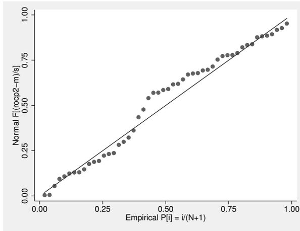
The closeness of the points to the horizontal line on the normal probability plot shows us that the bootstrap distribution is approximately normal. So it is reasonable to use the normal-based confidence intervals for ROC at a false-positive rate of 0.2 under covariate values  $xf = 10.01$ ,  $x1 = 6.5$ , and  $xd = 4$ .
