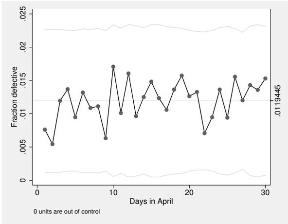
Here the control limits are, like the sample size, no longer constant. The `stabilize` option will stabilize the control chart:
