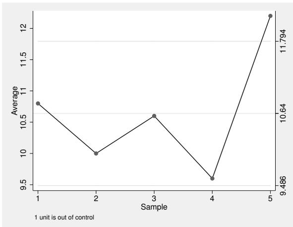
The average measurement in the sample is 10.64, and the lower and upper control limits are 9.486 and 11.794, respectively. Suppose that we knew from prior information that the mean of the process is 11. Then we would type
