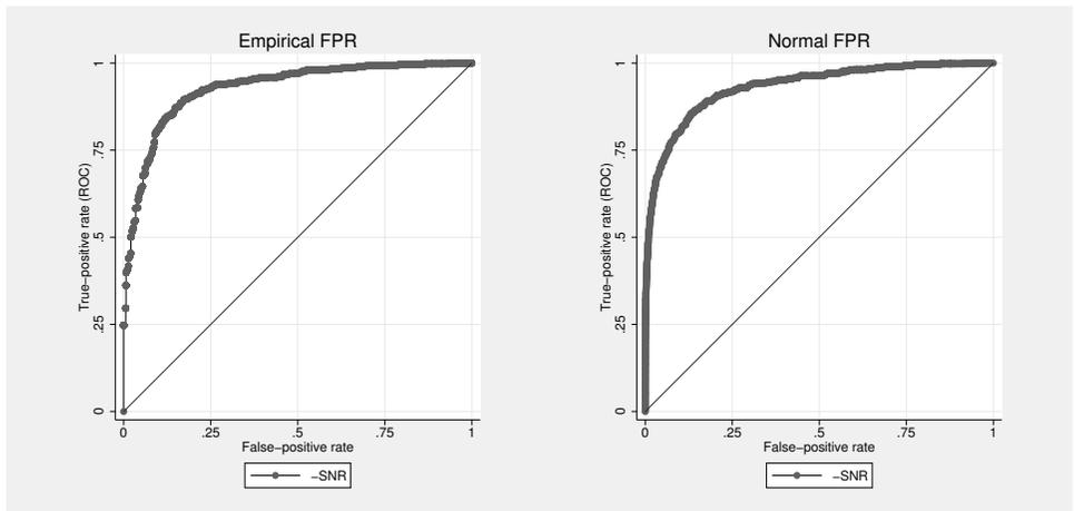
On cursory visual inspection, we see little difference between the two curves. The AUC values are close as well. So it is sensible to assume that we have Gaussian percentile values for control standardization. ◀
