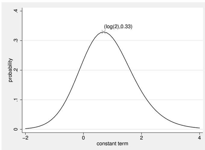
The lower and upper confidence bounds are the values of  $\theta$  such that  $\Pr(M \geq 4|\theta) = 0.025$  and  $\Pr(M \leq 4|\theta) = 0.025$ , respectively. These probabilities are plotted in the figure below for  $\theta \in [-2, 4]$ .
