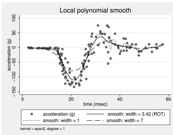
From this graph, we can see that the local linear polynomial fit with larger bandwidth (`width = 7`) corresponds to a smoother line but fails to fit the curvature of the scatterplot data. The smooth obtained using the width equal to one seems to fit most data points, but the corresponding line has several spikes indicating larger variability. The smooth obtained using the ROT bandwidth estimator seems to have a good tradeoff between the fit and variability in this example.
