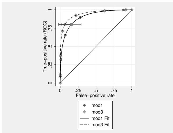
For estimation of the false-positive rate at a ROC value of 0.8, the confidence intervals overlap. Both classifiers require only a small false-positive rate to achieve a ROC value of 0.8.
