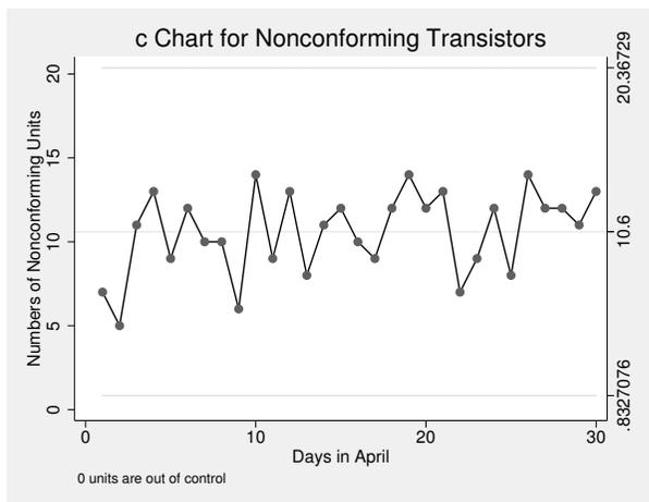
The expected number of defects is 10.6, with lower and upper control limits of 0.8327 and 20.37, respectively. No units are out of control.
