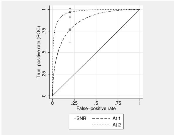
The ROC values are slightly higher at the false-positive rate of 0.2 than they were in the maximum likelihood estimation in [example 2](#). To see if the false-positive rates differ at a ROC value of 0.5, we specify the `invroc(.5)` option.
