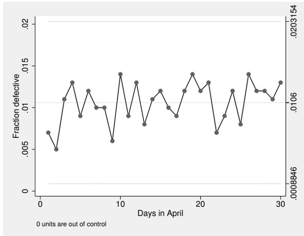
All the points are within the control limits, which are 0.0009 for the lower limit and 0.0203 for the upper limit.
