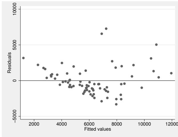
All the diagnostic plot commands allow the `graph twoway` and `graph twoway scatter` options; we specified a `yline(0)` to draw a line across the graph at  $y = 0$ ; see [G-2] [graph twoway scatter](#).
