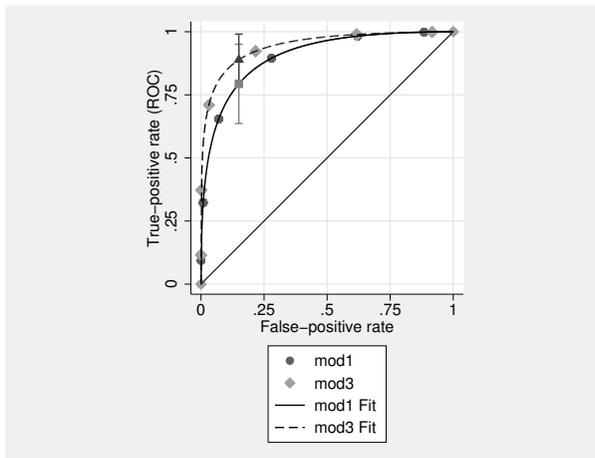
The ROC value for the false-positive rate of 0.15 is more separated in the two classifiers. Here we see that mod3 has a larger ROC value than mod1 for this false-positive rate, but the confidence intervals of the estimates overlap.
