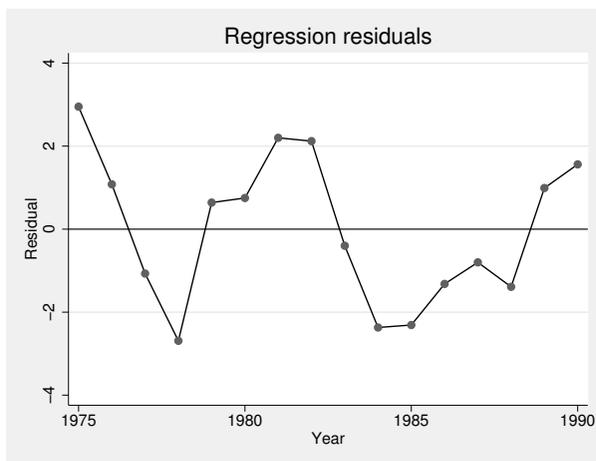
The graph gives the impression that these residuals are positively correlated. Excursions above or below zero—the natural threshold for regression residuals—tend to last for several observations. `runtest` can evaluate the statistical significance of this impression.
