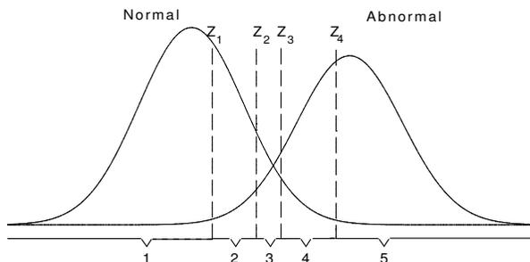
The latent variable is assumed to be normally distributed for both the normal and abnormal subjects, perhaps after a monotonic transformation, with means  $\mu_n$  and  $\mu_a$  and variances  $\sigma_n^2$  and  $\sigma_a^2$ , respectively.
